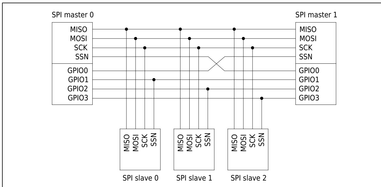
Figure 18-6 Schematic diagram of SPI multi-master/multi-slave system
